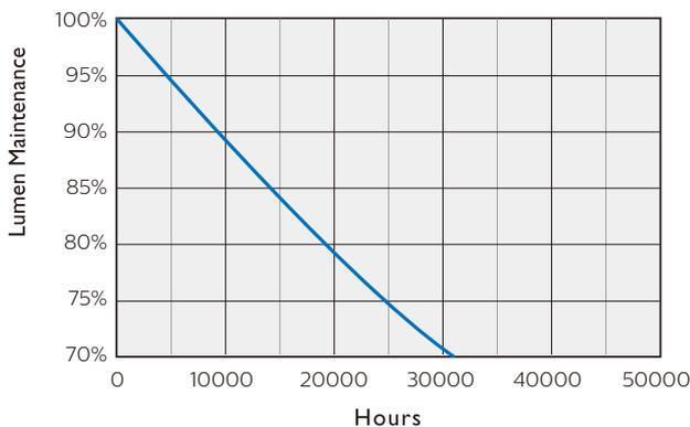
Philips Essential LEDtube has a lifetime of 30,000 hours, defined as the number of hours when 50% of a large group of identical lamps below 70% of its initial lumens.
